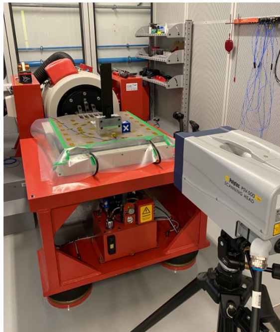
Fig. 2 Ground vibration test of an experimental blade.
