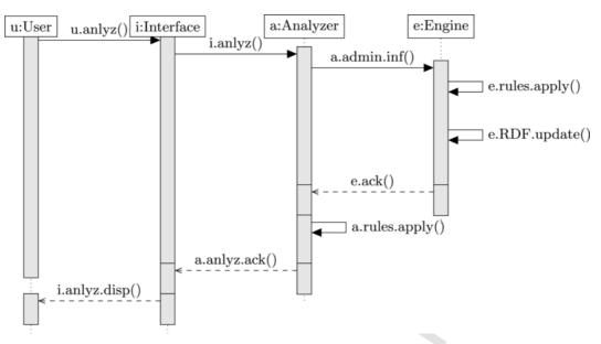
Fig. 16. The sequence diagram for the administration analysis.
