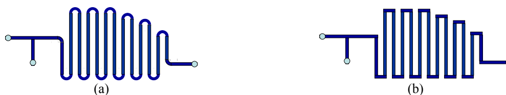
Figure 1: Microchannel geometries used in this study with w = 1000 \mu\text{m} , h = 500 \mu\text{m} and l \approx 30 \text{ cm} . (a) Curved meandering channel, (b) angled meandering channel.
