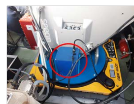
Figure 3 : Left : IMAO PA03 airplane, Right : SIMAGAZ instrument (blue inside the red circle) integrated in the airborne stabilised platform.
