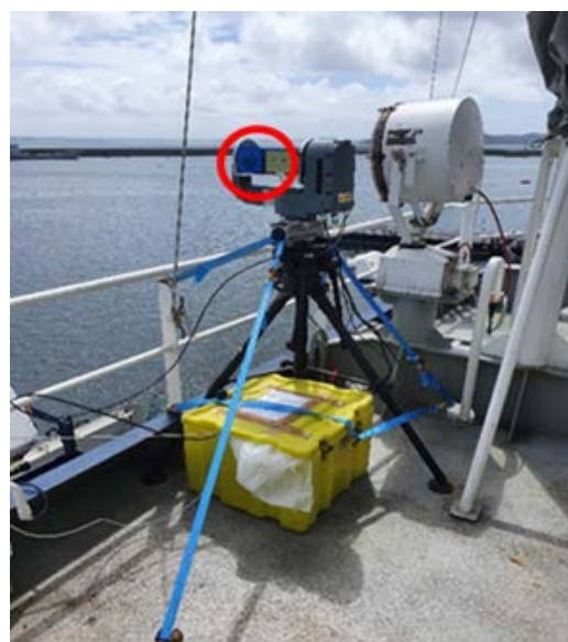
Figure 2: SIMAGAZ instrument (blue one in the red circle) integrated on a stabilised platform on-board CEPOL vessel during the experiment.
