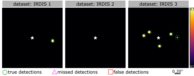
Figure 10. Detection maps obtained with the proposed algorithm on the three SPHERE-IRDIS datasets from the EIDC data challenge, see Sect. 4 for the observation logs. Sources are classified as true, missed and false detections. The detection threshold is set to \tau = 0.5 .
