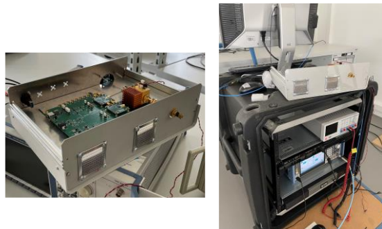
Fig. 2. Transmitter front-end (left) and rack (right)
