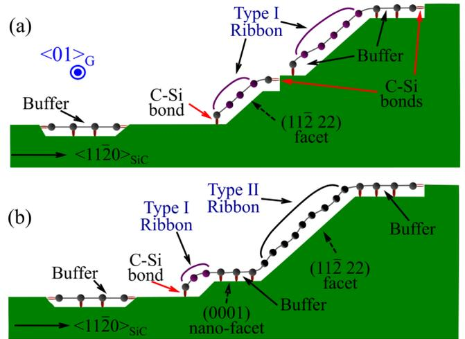
FIG. 7. Two edge-terminated  $6H$  ZZ ribbons. Functionalized (buffer) graphene is represented by gray circles bonded to the SiC. (a) Type I ribbons terminated by C-C bonds into buffer graphene on one side and C-Si bonds to the substrate on the other side. (b) A type II termination with metallic graphene terminated on both sides by C-C bonds into buffer graphene.
