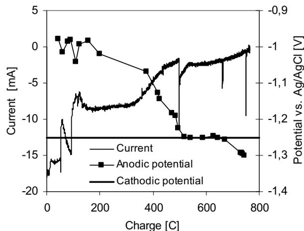
**Fig. 3** Evolution of anodic potential and current during the potentiostatic electrolysis (run 5)
