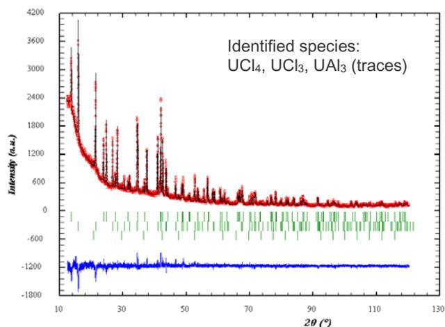
**Fig. 8** XRD pattern of the chlorination product (Symbols = observed points, solid line above = calculated profile, solid line below = difference between observed and calculated profiles, ticks below the peaks =  $2\theta_{hkl}$  Bragg positions for  $\text{UCl}_4$ ,  $\text{UCl}_3$  and  $\text{UCl}_3$ , in descending order)
