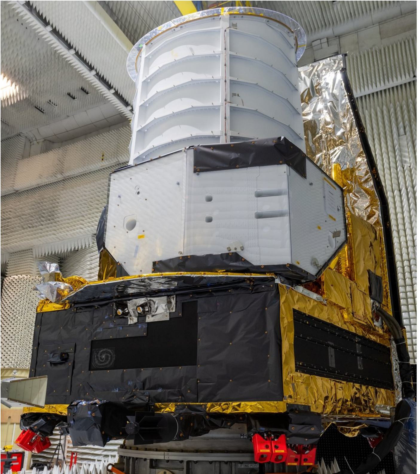
Fig. B.5. Fully assembled spacecraft on February 2023 in the anechoic chamber of Thales Alenia Space in France, after completing final electromagnetic compatibility (EMC) tests. The side shown here will always face away from the Sun. The hydrazine thrusters on the SVM still have their protective red covers on, and point away from the PLM to minimise contamination in flight (see Sect. 4.6.4). The plaque with the miniaturised fingerprint galaxy created by Euclid Consortium members can be seen at the lower left of the SVM ( https://www.esa.int/ESA_Multimedia/Videos/2022/07/The_Fingertip_Galaxy_Reflecting_Euclid_in_art ). A high-resolution image is available at https://www.esa-photolibrary.com/ESA/media/73223 . Credit: ESA - M. Pédoussaut.
