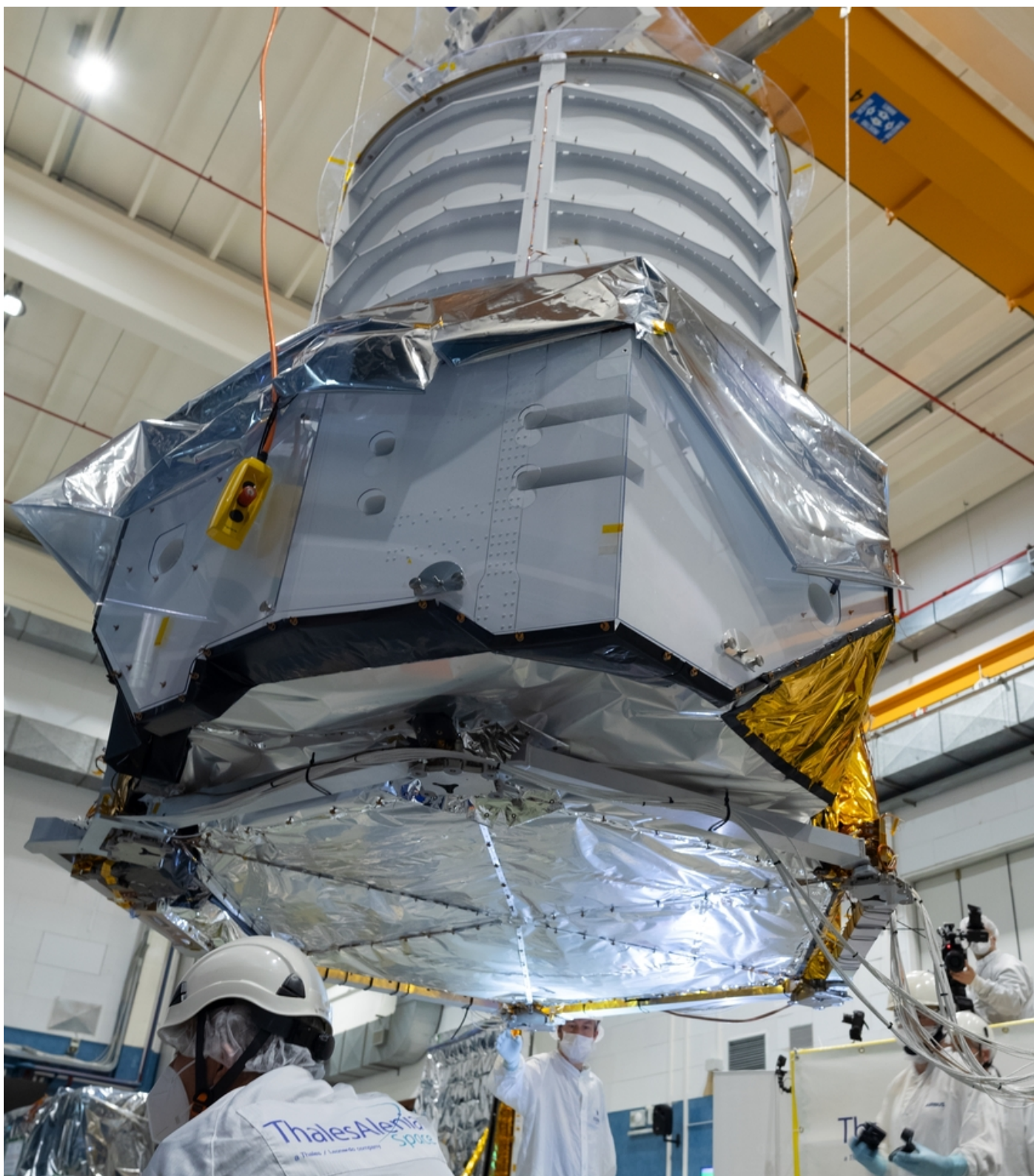
Fig. B.4. Bottom of the PLM, shortly before the mating with the SVM shown in Fig. B.3. The bottom is covered with MLI to provide thermal insulation and to prevent molecular contamination entering from the SVM. The large white polygonal structure girding the lower parts is the NISP radiator. A high-resolution image is available after account creation from the ESA Photo Library For Professionals at https://www.esa-photolibrary.com/ESA/media/65700 . The PLM was built by Airbus Defence and Space. Credit: ESA - S. Corvaja.
