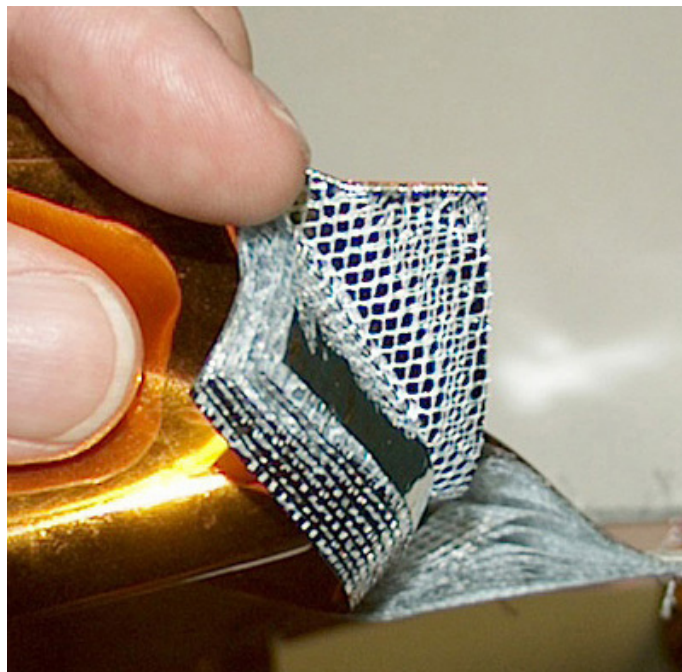
Fig. 1. Structure of a MLI thermal blanket, the main source of water contamination in spacecraft. Figure credit: John Rossie of Aerospace Educational Development Program (AEDP), CC BY-SA 2.5 license.
