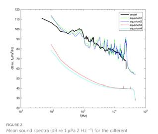
Mean sound spectra (dB re 1  $\mu$ Pa 2 Hz  $^{-1}$ ) for the different experiments. Bold black line represents the vessel noise recorded *in situ* and the other lines of the spectra of sounds recorded in the four tanks used. Green and blue lines are from tanks 1 and 2 for the sound treatment and red and light-blue lines are from tanks 3 and 4 for the silent treatment.
