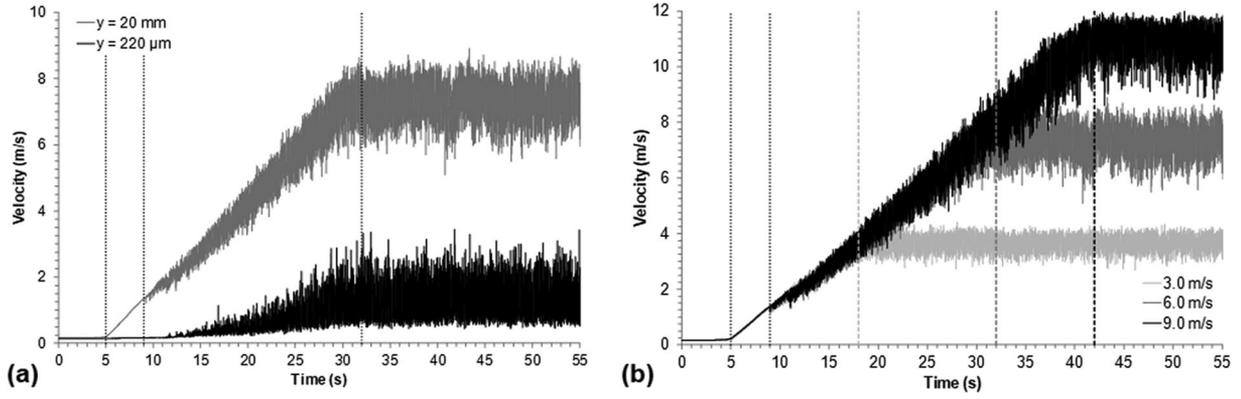
**Figure 3.** Temporal evolution of the velocity: (a) at the half duct height ( $y = 20$  mm) and in the viscous sublayer ( $y^+ = 4.1$ , i.e.,  $y = 220$   $\mu\text{m}$ ) for  $U_{\text{mean}} = 6.0 \text{ m}\cdot\text{s}^{-1}$  and  $\alpha_{\text{mean}} = 0.3 \text{ m}\cdot\text{s}^{-2}$ ; (b) at the half duct height ( $y = 20$  mm) for  $U_{\text{mean}} = 3.0$ ; 6.0 and  $9.0 \text{ m}\cdot\text{s}^{-1}$  and  $\alpha_{\text{mean}} = 0.3 \text{ m}\cdot\text{s}^{-2}$ .
