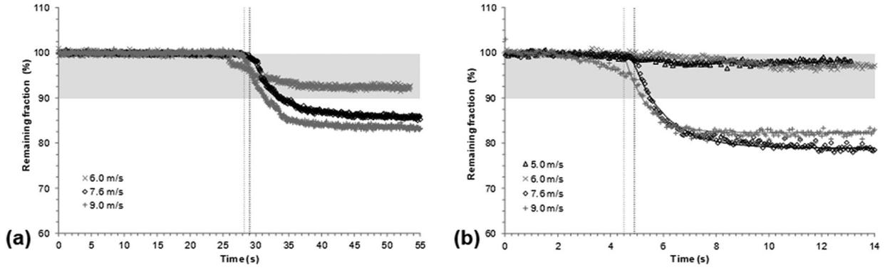
**Figure 5.** Temporal evolution of the remaining fraction: (a) for  $U_{\text{mean}} = 6.0; 7.6$  and  $9.0 \text{ m.s}^{-1}$  and  $\alpha_{\text{mean}} = 0.3 \text{ m.s}^{-2}$ ; (b) for  $U_{\text{mean}} = 5.0; 6.0; 7.6$  and  $9.0 \text{ m.s}^{-1}$  and  $\alpha_{\text{mean}} = 2.1 \text{ m.s}^{-2}$ .
