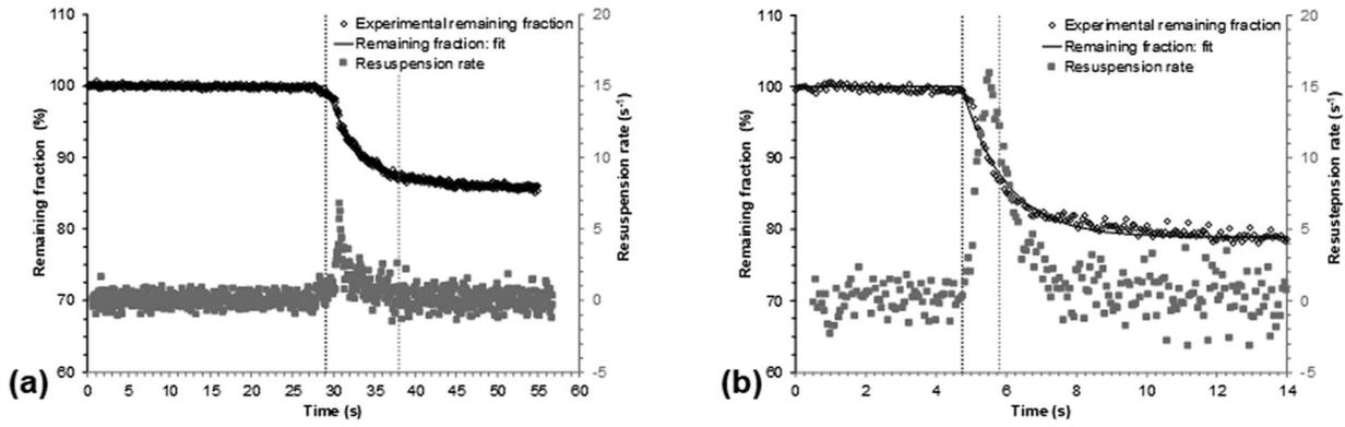
**Figure 8.** Temporal evolution of the remaining fraction versus temporal evolution of the resuspension rate for  $U_{\text{mean}} = 7.6 \text{ m.s}^{-1}$ : (a) for  $\alpha_{\text{mean}} = 0.3 \text{ m.s}^{-2}$ ; (b) for  $\alpha_{\text{mean}} = 2.1 \text{ m.s}^{-2}$ .
