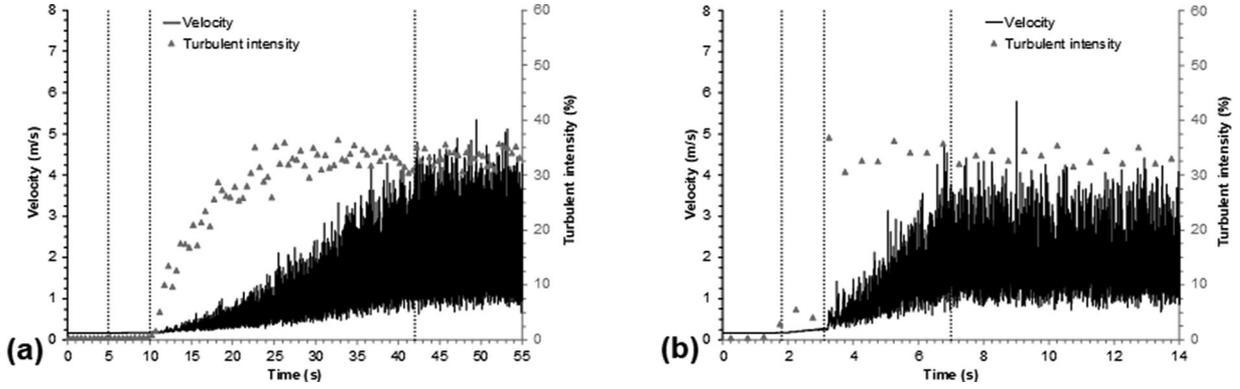
**Figure 4.** Temporal evolution of the velocity and the turbulent intensity in the viscous sublayer: (a) for  $U_{mean} = 9.0 \text{ m.s}^{-1}$  and  $\alpha_{mean} = 0.3 \text{ m.s}^{-2}$  ( $y = 180 \mu\text{m}$ ); (b) for  $U_{mean} = 9.0 \text{ m.s}^{-1}$  and  $\alpha_{mean} = 2.1 \text{ m.s}^{-2}$  ( $y = 160 \mu\text{m}$ ).
