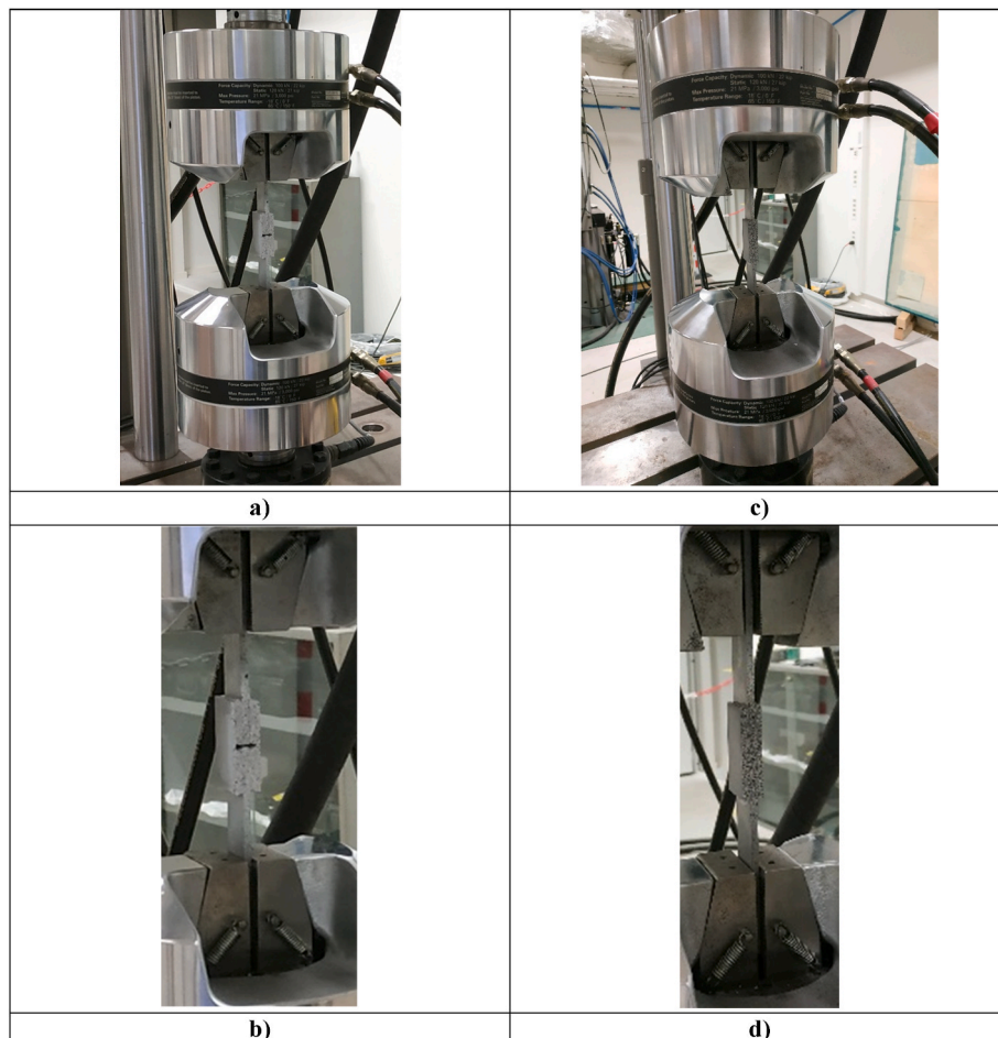
Fig. 5. Double lap shear tests for different adhesive thicknesses: a-b) 4 mm and c-d) 2 mm.
