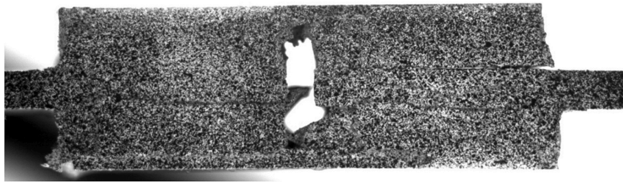
Fig. 9. Detailed view of the failed adhesive region of the test M4#12.
