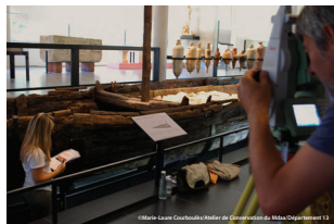
Topographical survey (11 reference points ; 160 control points)
