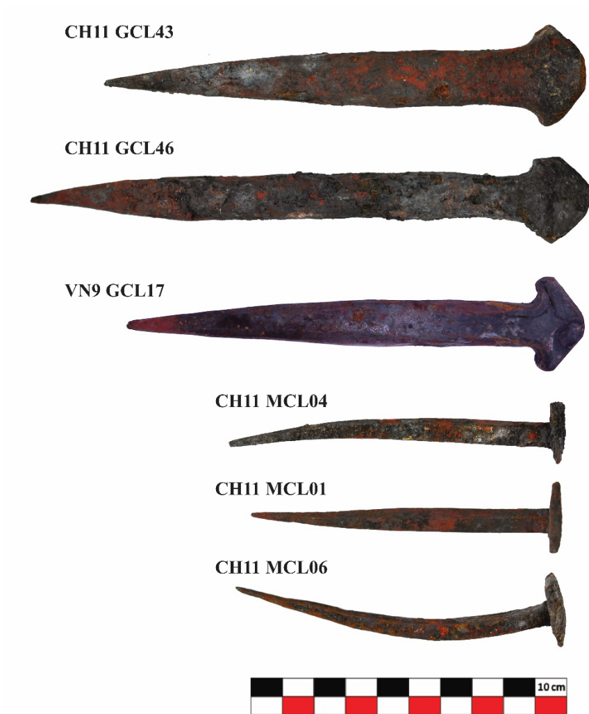
Figure 4: Different types of forged nails found in the excavation of the vaults debris.
