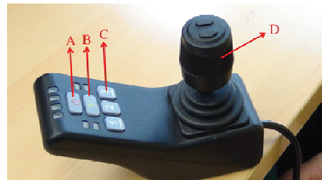
A = On/off push button B = Home position push button C = Push buttons 1, 2 and 3 D = Shaft ring
