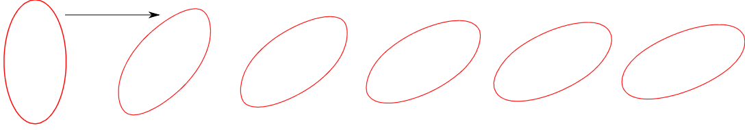
FIGURE 5: TT regime for \Xi_{2d} = 0.68 , \beta = 1 , Ca = 4 \times 10^4 and Re = 9 \times 10^{-3} at t \in \{0, 0.125, 0.25, 0.5, 1, 2\} .
