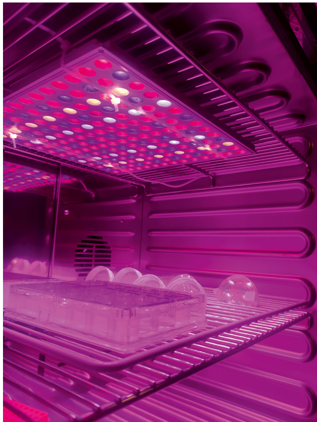
Figure 1. Peltier cooled incubator to grow Arabidopsis thaliana seedlings
