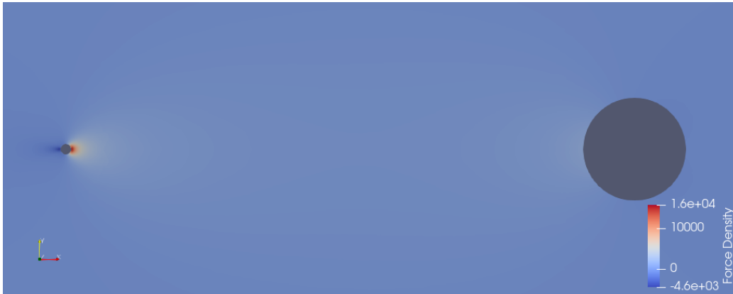
Figure 12: EHD force density F_x ( Nm^{-3} ) at T = 4ms for r_1 = 0.1mm , d = 10mm , V_G = 13kV , \psi = 10^{10}m^{-3} (figure reflected on symmetric boundaries)
