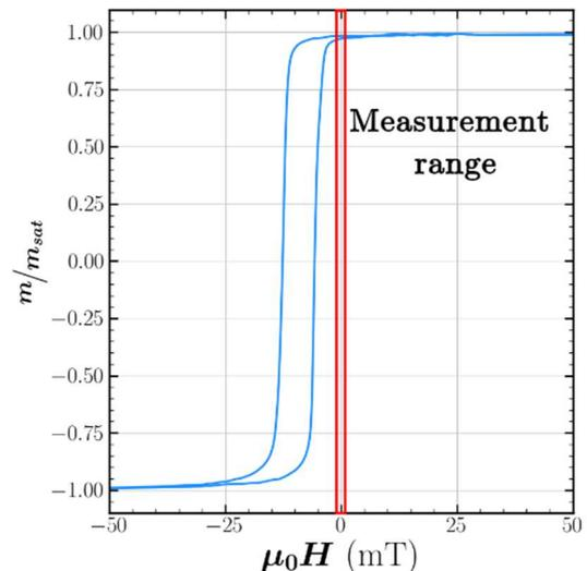
Figure 6. Hysteresis loop of the NiMn/CoFe stack
