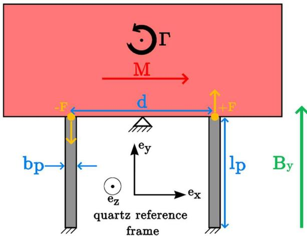
Figure 1. Working principle of the resonator
