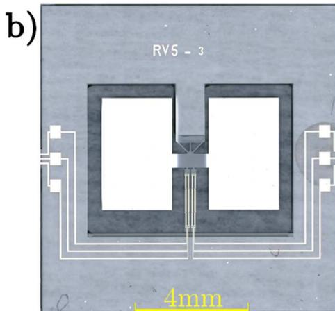
Figure 4. a) Fabrication process of a resonator b) Realisation of a resonator with magnetic materials on the plates
