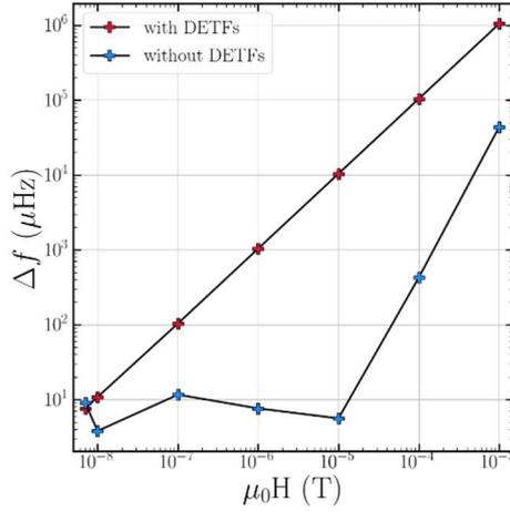
Figure 2. Simulated  $\Delta f = f(B_y)$  for resonators with and without DETFs
