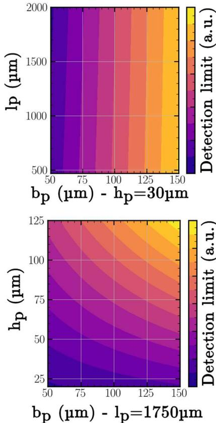
Figure 3. Detection limit as a function of  $b_p$ ,  $l_p$  and  $h_p$
