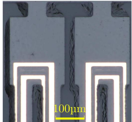
Figure 5. Side-walls around the top heads of the DETFS
