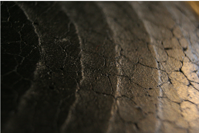
Figure 1: Close up of the syahi. The reticulum of cracks and different layers can be seen
