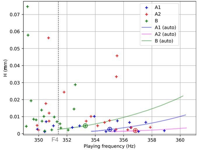
Figure 16: Variation of  $H$  as a function of  $F_{play}$ . Crosses represent the measures for all three musicians, circles the initialization parameter for continuation (see section 2.9), and lines the continuation obtained with auto-07p. The dashed line represents the average frequency of the actual played F4 with no bend.
