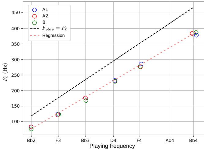
Figure 6: Variation of  $F_{\ell}$  as a function of  $F_{play}$  for all three musicians in circles, together with the diagonal  $F_{play} = F_{\ell}$  in dashed black, and the regression line in dashed red.
