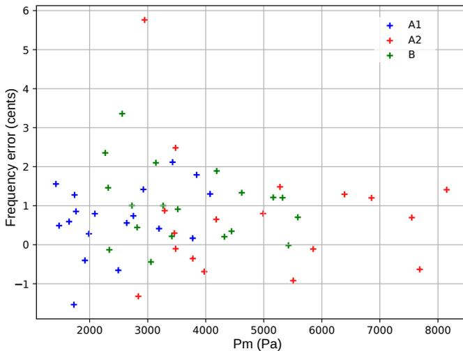
Figure 19: Variation of frequency error as a function of  $P_m$  for all three players.
