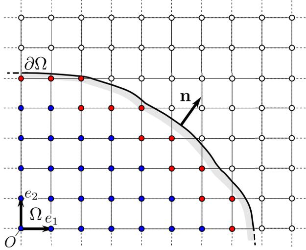
Figure 2: Lattice nodes classification, for  $d = 2$ , with in blue the nodes of  $\mathcal{I}_{\text{in}}$ , in red the nodes of  $\mathcal{I}_{\text{bd}}$  and in white the nodes that are not considered.
