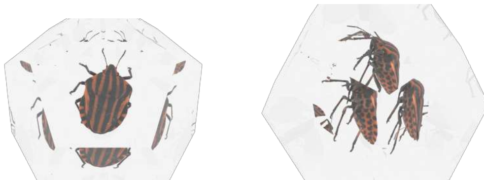
Figure 15. Two images of the graphosoma immersed in a regular dodecahedron of epoxy resin.
