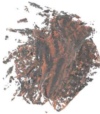
Figure 19. 3D reconstruction by MVS, from 18 images such as those in Figure 17: the result looks like a random 3D point cloud.
