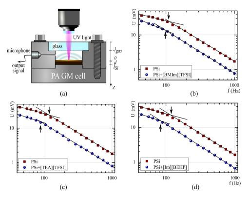
**Figure 3.** PA cell with gas-microphone registration employed (**a**), amplitude-frequency characteristics of PSi and "PSi/IL" composite systems with IL: [BMIm][TFSI] (**b**), [TEA][TFSI] (**c**), [Im][BEHP] (**d**). Arrows indicate the bending frequency.
