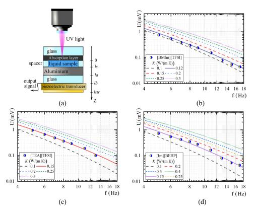
**Figure 2.** PA cell with piezoelectric registration employed (a), amplitude-frequency characteristics of a multilayer system with IL: [BMIm][TFSI] (b), [TEA][TFSI] (c), [Im][BEHP] (d). Circles indicate the experimental data, lines—the simulation of PA signal formation at different values of thermal conductivity of the liquid sample.
