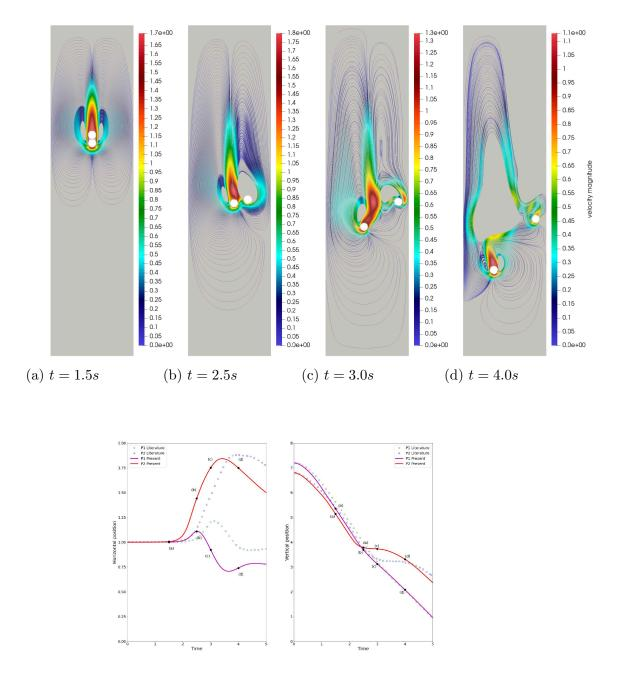
Figure 5: The upper figures show the position of the two disks as well as the streamlines at four different time instants. The lower graphs compare the evolution of the disks horizontal and vertical position to literature [24]. The solid lines correspond to present results and the dotted one to literature results.
