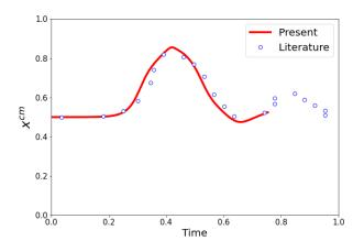
Figure 4: Evolution of the horizontal position of the center of the ellipsoid. The dotted line shows the literature results [23] and the red line represents the present results.
