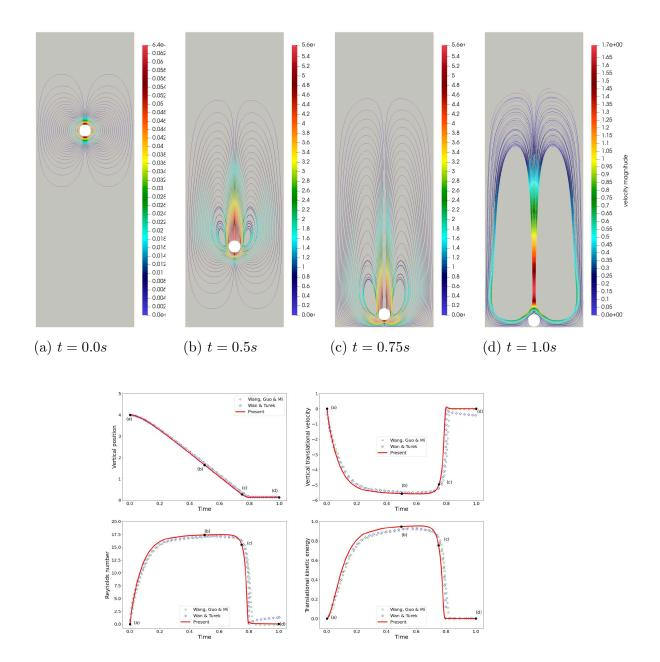
Figure 1: Evolution of the vertical position of mass center, vertical translational velocity, Reynolds number and translational kinetic energy. The red line are the present results, the green dotted and blue dotted lines correspond to results respectively taken from [19] and [18]. The streamlines and body position at four different time instants are represented.
