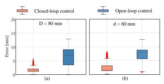
Fig. 10. Results for Experiment 3: Summarised tracking errors for (a) a circle with a diameter of 80 mm, (b) rectangle with a side length of 60 mm.
