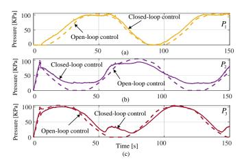
Fig. 11. Comparison of pressure values for open- and closed-loop control for the one-module robot following a 40 mm-diameter circular trajectory.
