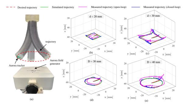
Fig. 7. Results for Experiment 2: Trajectory tracking performance of open-loop and the closed-loop control. (a) Measurement of the robot's trajectory. Results for (b) tracking a rectangle, with a side length of 20 mm, (c) tracking a rectangle, with a side length of 30 mm, (d) tracking a circle, with a diameter of 30 mm, and (e) tracking a circle, with a diameter of 40 mm.
