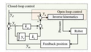
Fig. 5. The open-loop and closed-loop control scheme.  $y_d$  is the desired position,  $y_u$  is the input position to the inverse controller, and  $y_m$  is the measured position. For open-loop control,  $y_u$  equals  $y_d$  without feedback correction. While  $y_u$  is compensated by the feedback position using a PI controller in the closed-loop control.
