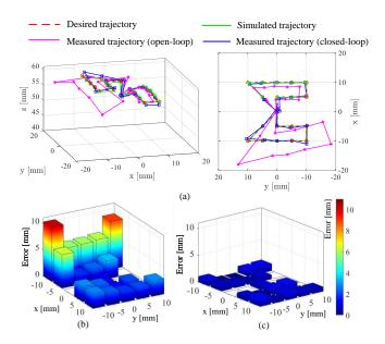
Fig. 6. Results for Experiment 1: (a) Comparison between the measured tip position, the simulated position and the desired position for the open-loop and closed-loop controller. The summarised mean absolute tip errors with respect to different desired points are shown in (b) and (c).
