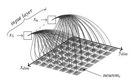
Fig. 2 Kohonen feature map network. (The connections between the input and output layers indicate the relationships between the input and output vectors.)
