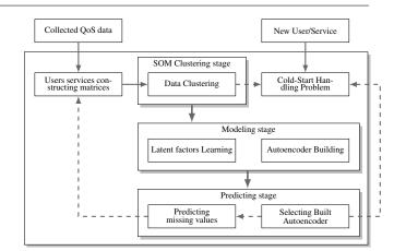
Fig. 3 Overview of the prediction system architecture
