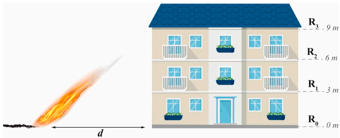
Figure 4. Configuration of the “building” target with respect to the flame front position.
