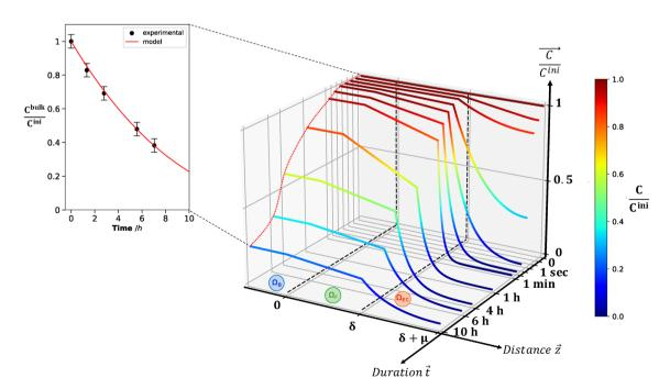
**FIGURE 6** Spatio-temporal profiles of the urea concentration during a potentiostatic electrolysis at 0.55 V of a 0.33 mol L<sup>-1</sup> urea solution in alkaline media (5 mol L<sup>-1</sup> KOH), on nickel massive electrode. Inset: dimensionless urea concentrations in the bulk  $\Omega_B$  measured experimentally (black filled circles) and predicted by the m odel (red line).
