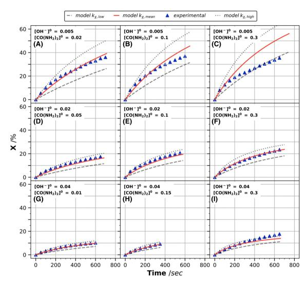
**FIGURE 2** Comparison of the experimental temporal evolutions of the hydroxide ion conversion to the ones obtained by numerical solving of Equation (22) for different initial concentrations of urea and hydroxide (molar concentration are expressed in mol  $L^{-1}$ ). The surface accessibility factor of nickel(III),  $\varepsilon$ , is equal to 2.6% whatever the graphs.
