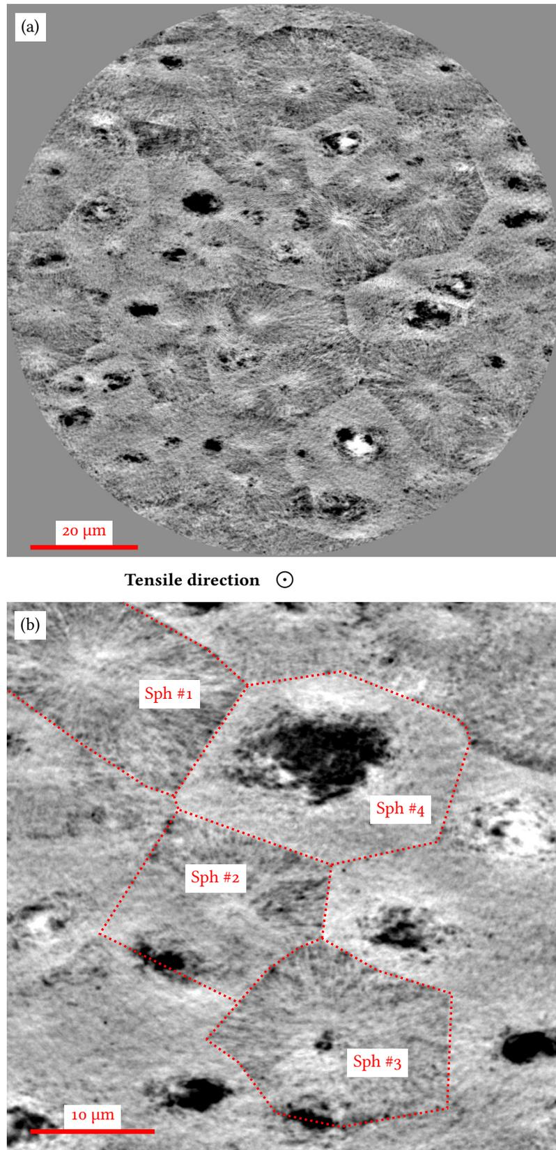
**Figure 7** Top views of data set of deformed PP at a resolution of 50 nm: (a) global view  $102\ \mu\text{m} \times 102\ \mu\text{m}$ ; (b) closer look at few spherulites:  $45\ \mu\text{m} \times 45\ \mu\text{m}$ .
