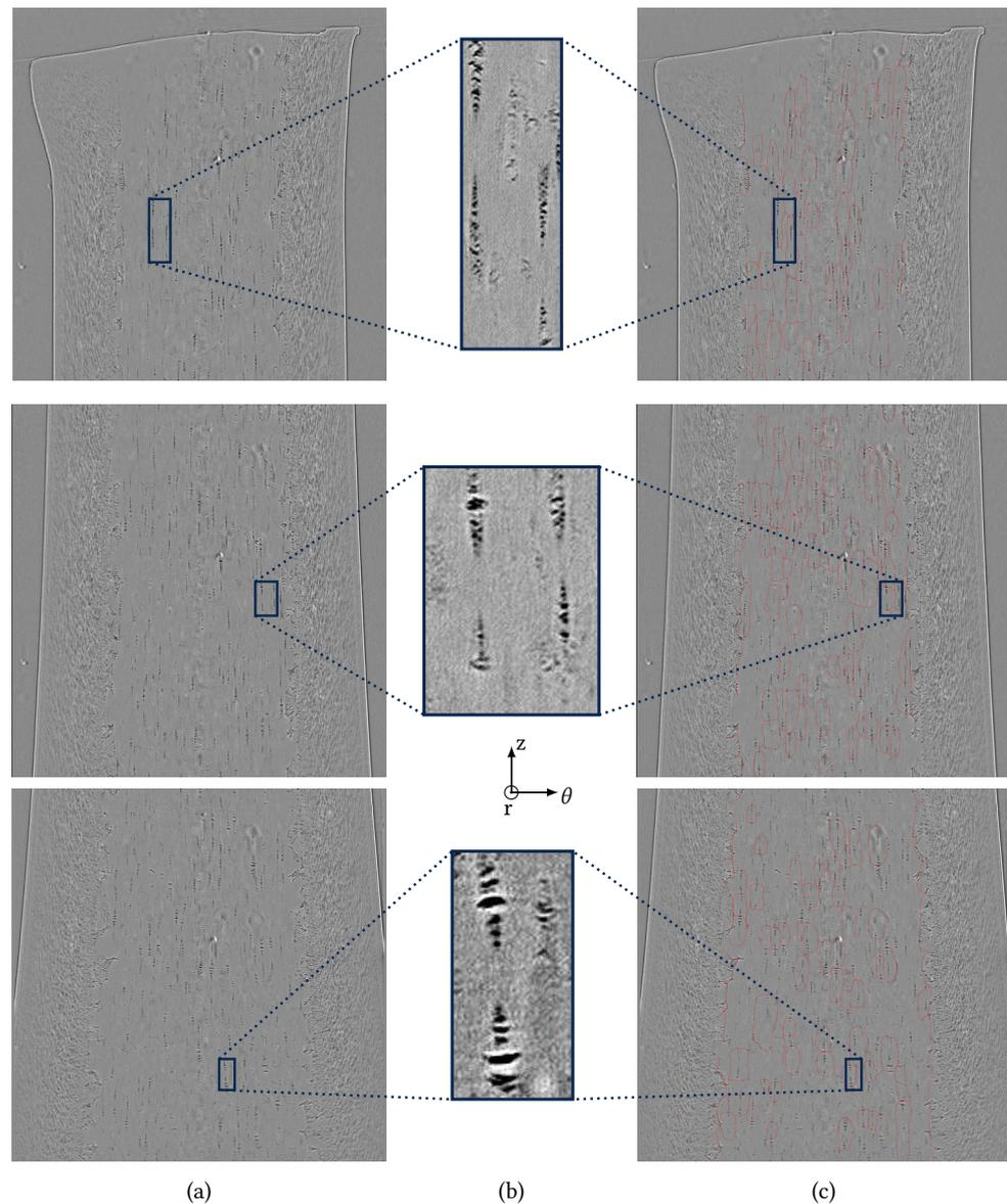
**Figure 9** Side views of the three VOIs presented in Figure 3 so as to determine the heights of the deformed spherulites: (a) Reconstructed images; (b) Closer examinations of a specific region; (c) Drawings of the identified polar fans inside the deformed spherulites.
