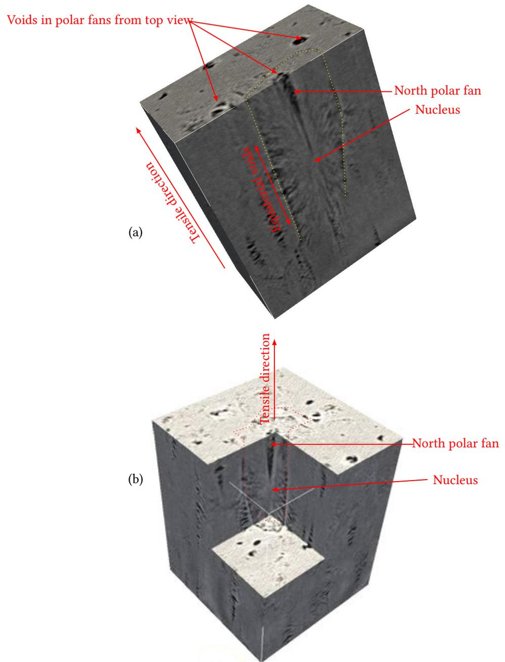
**Figure 5** Various 3D views of deformed spherulites showing polar fans, from data sets obtained from Synchrotron Radiation Tomography with a resolution corresponding to  $1 \text{ px} \approx 0.7 \mu\text{m}$ . Cube side about  $140 \mu\text{m}$ .
