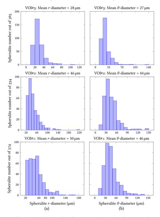
**Figure 10** Histograms of the diameters of the identified deformed spherulites in the core, for VOIs#1,2,3 from bottom to top: (a) diameter along r-direction; (b) diameter along  $\theta$ -direction (See Figure 8 for the cylindrical coordinates).
