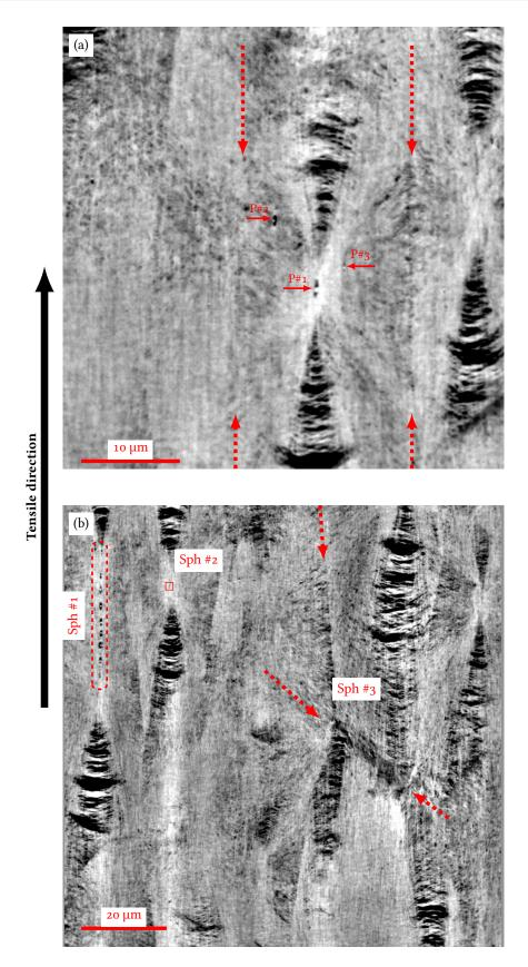
Figure 6 Side views of the data set of deformed PP at a resolution of 50 nm: (a) detailed view of a couple of polar fans; (b) global view  $102 \, \mu m \times 102 \, \mu m$ .
