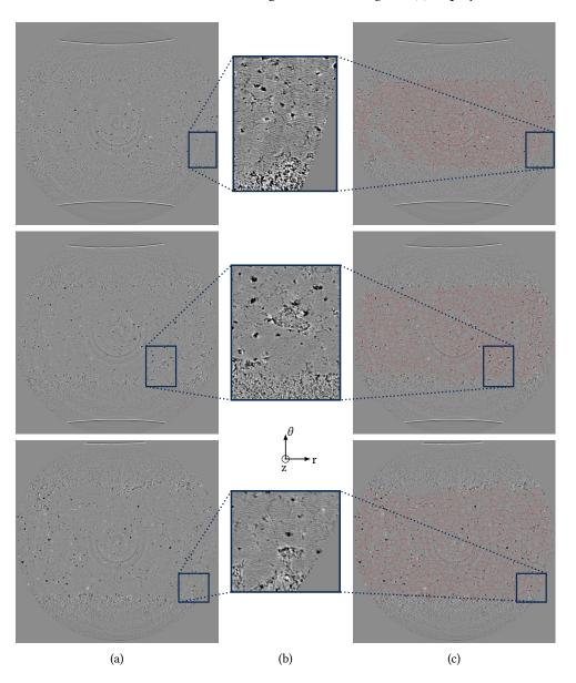
**Figure 8** 2D section top views of microtomography data of the three VOIs presented in Figure 3 so as to determine the diameters of the deformed spherulites: (a) Reconstructed images; (b) Closer examinations of a specific region; (c) Drawings of the identified boundaries for the deformed spherulites.
