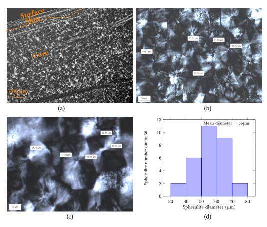
Figure 2 Optical microscopy examination of the spherulites on microtomed thin film of the PP under study: (a) Large surface; (b) and (c) Focuses on smaller surfaces to allow diameter measurements; (d) Histogram of the spherulite diameter measured on 30 net spherulites.
