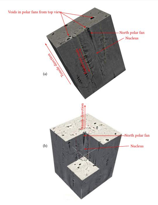
Various 3D views of deformed spherulites showing polar fans, from data sets obtained from Synchrotron Figure 5 Radiation Tomography with a resolution corresponding to 1 px  $\approx 0.7 \mu m$ . Cube side about 140  $\mu m$ .
