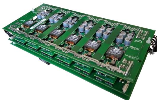
**Fig. 3** PCA prototype with 12 CSCs (6 series of 2 cells parallels) used to characterize the impact of interleaving driving signals on conducted EMI disturbances.
