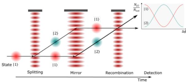
**FIG. 4.** The Mach-Zehnder configuration uses a series of three pulses: the first pulse separates the atomic wave, the second redirects the two partial waves, and the final pulse causes the two wavepackets to recombine and interfere. The interference is detected, for example, by measuring the number of atoms in one of the output states.
