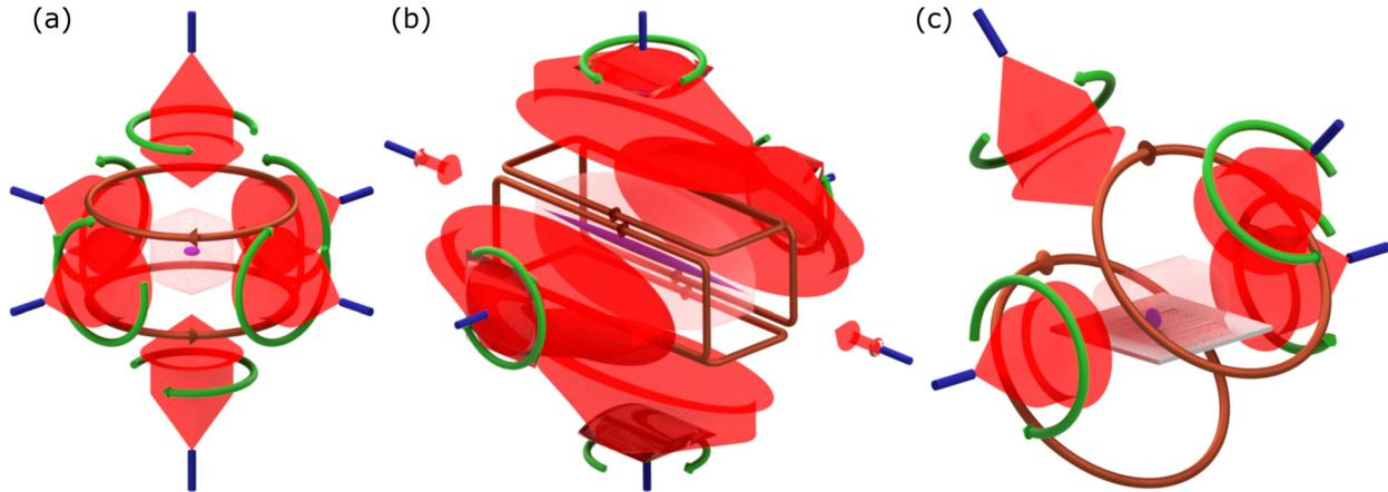
**FIG. 9.** Magneto-optical trap geometries: six-beam 3D MOT (a), a 2D(+) MOT (b), and reflection 3D MOT (c). The blue fibers deliver cooling and repumping light (red) which is collimated by lenses and appropriately circularly polarized (green arrows) with quarter-wave plates. Beam overlap regions are in light red, with MOT shape in purple. The vacuum pump, cell, and atom source are omitted for clarity, but anti-Helmholtz magnetic coils and current flow are indicated (copper).
