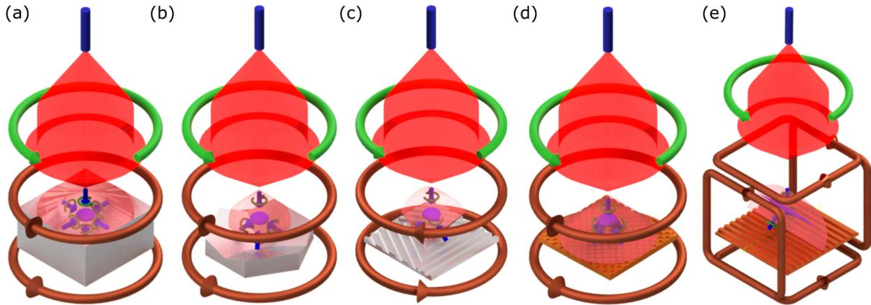
**Fig. 10.** Compact single-input-beam magneto-optical trap geometries, with Fig. 9 color scheme: pyramid MOT (a), tetra-pyramid MOT (b), 3D “triangle” grating MOT (c), 3D “checkerboard” grating MOT (d), and 2D grating MOT (e) as described in Ref. 132. In all geometries except (a) some of the beam overlap is above the pyramid/grating optic, which can be used *ex vacuo*. The vacuum pump, cell, and atom source are omitted for clarity.
