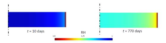
Fig. 5. Simulated relative humidity fields at two different times: at t=10 days (left), and at t=770 days (right).
