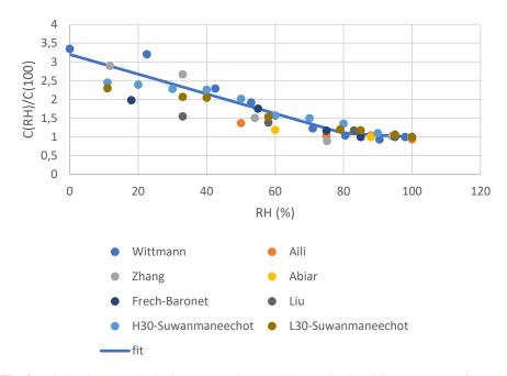
**Fig. 3.** Relation between the basic creep modulus and the relative humidity (creep tests from [2, 3 and 14], micro-indentation tests from [10, 11, 12, 13]).
