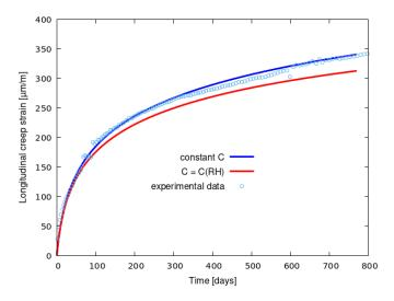
**Fig. 6.** Evolution of the longitudinal creep strain: (a) with the RH-independent creep model (blue curve), and (b) with the RH-dependent model as given by Eq. (2) (red curve).
