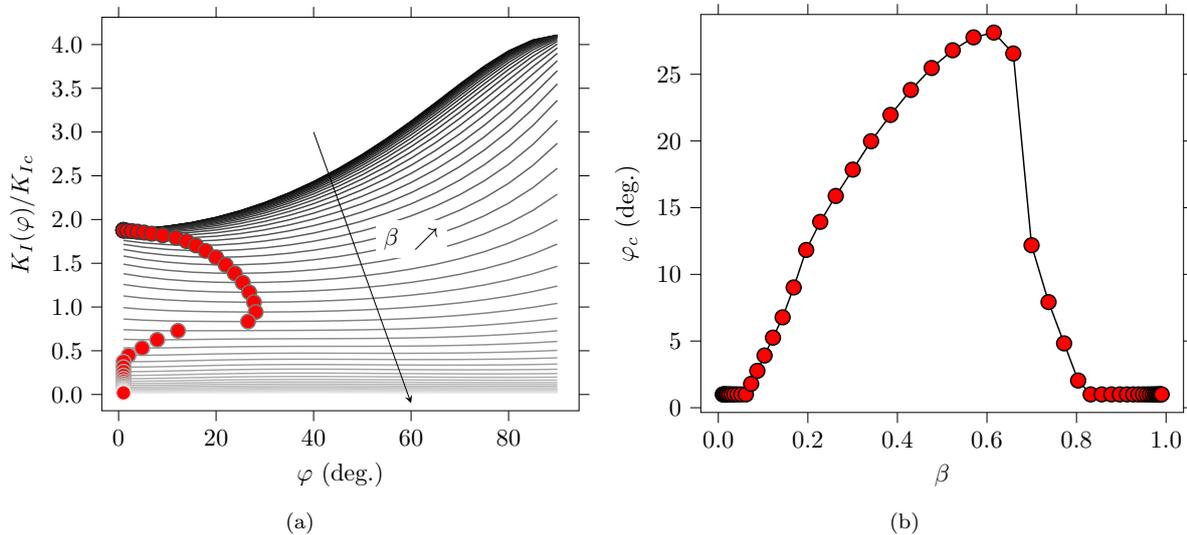
Fig. 5: a) Normalized facet nucleation SIF as a function of the facet angle for several mode mixities (circles represent the facet nucleation apparent SIF, *i.e.* the minimum SIF for a given mixity) and b) Initiation facet angle (minimizing normalized facet nucleation SIF) as a function of the mode mixity.
