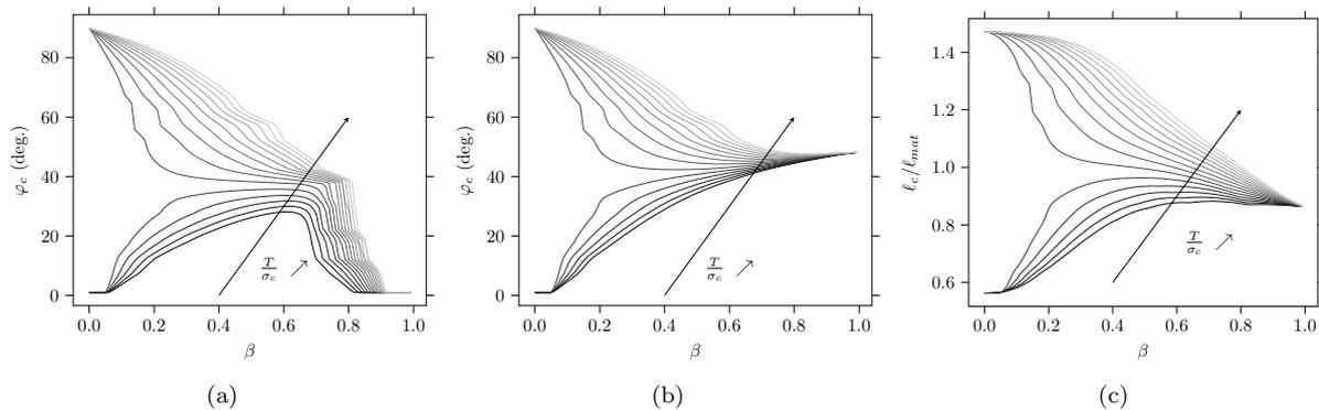
Fig. 15: a-b) Facet nucleation angle and c) normalized initiation length as a function of the mode mixity for different T-stress magnitudes for a)  $\mathcal{G}_{IIIc}/\mathcal{G}_{Ic} = 1$ , and b-c)  $\mathcal{G}_{IIIc}/\mathcal{G}_{Ic} = 10$ .
