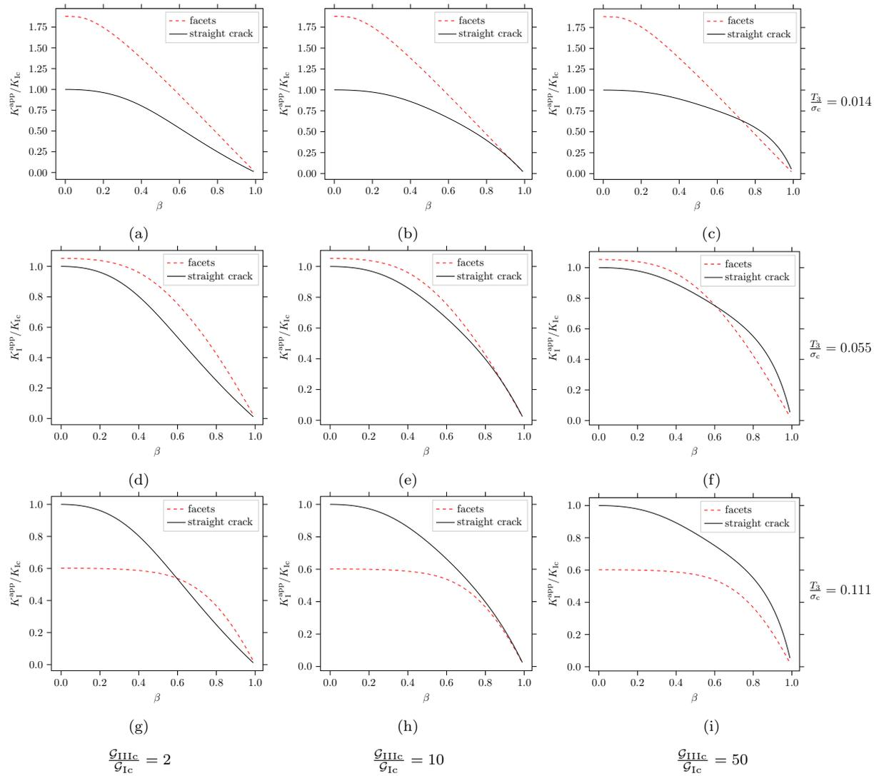
Fig. 16: Normalized facet nucleation (dashed line) and straight crack propagation (plain line) apparent SIF as a function of the mode mixity obtained for a-c)  $T_3/\sigma_c = 0.014$  d-f)  $T_3/\sigma_c = 0.055$  and g-i)  $T_3/\sigma_c = 0.111$  and a,d,g)  $\mathcal{G}_{IIIc}/\mathcal{G}_{Ic} = 2$ , b,e,h)  $\mathcal{G}_{IIIc}/\mathcal{G}_{Ic} = 10$  and c,f,i)  $\mathcal{G}_{IIIc}/\mathcal{G}_{Ic} = 50$ .
