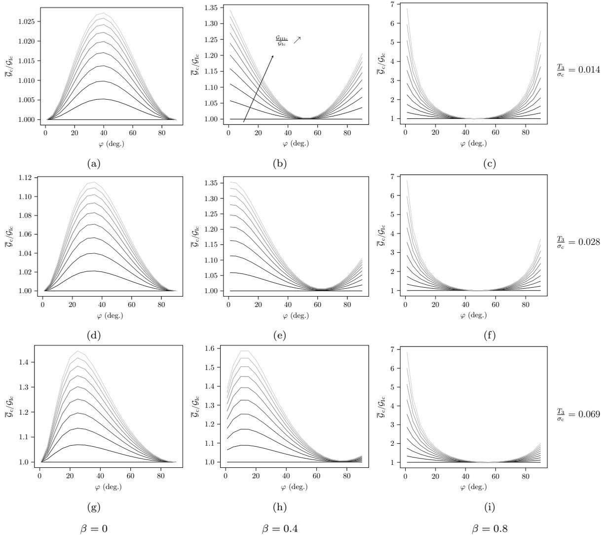
Fig. 13: Normalized average critical ERR as a function of facet angle obtained for  $\mathcal{G}_{IIIc}/\mathcal{G}_{Ic}$  ratios between 1 and 50, a-c)  $T_3/\sigma_c = 0.014$ , d-f)  $T_3/\sigma_c = 0.028$  and a-c)  $T_3/\sigma_c = 0.069$  normalized T-stress magnitudes and a,d,g)  $\beta = 0$ , b,e,h)  $\beta = 0.4$  or c,f,i)  $\beta = 0.8$  mode mixities.
