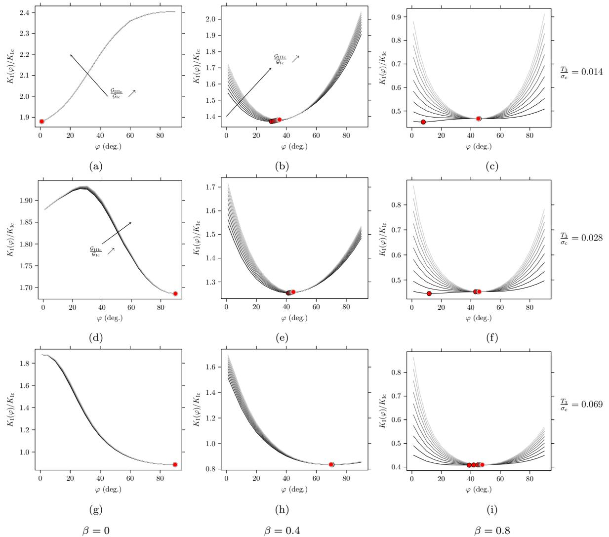
Fig. 14: Normalized facet nucleation SIF variation as a function of facet angle obtained for  $\mathcal{G}_{IIIc}/\mathcal{G}_{Ic}$  ratios between 1 and 50, for a-c)  $T_3/\sigma_c = 0.014$ , d-f)  $T_3/\sigma_c = 0.028$  and a-c)  $T_3/\sigma_c = 0.069$  normalized T-stress magnitudes and a,d,g)  $\beta = 0$ , b,e,h)  $\beta = 0.4$  or c,f,i)  $\beta = 0.8$  mode mixities.
