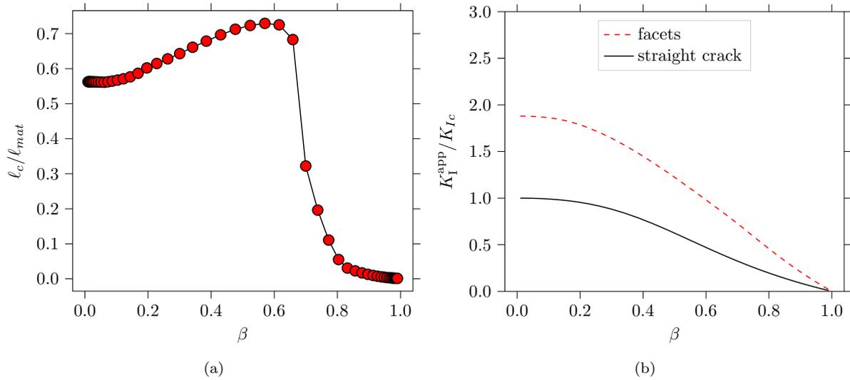
Fig. 6: Normalized a) initiation facet extension along ( $Ox_1$ ) direction and b) apparent SIF corresponding either to facet nucleation (dashed line) or straight crack propagation (plain line) as a function of the mode mixity.
