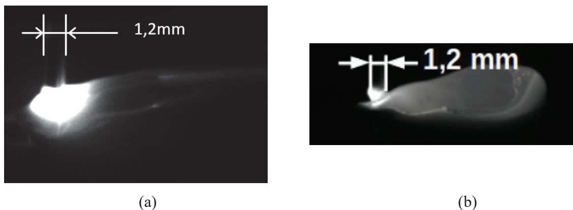
Figure 1: Comparison of the melt pool image measured with a CMOS camera in function of the material, (a) Aluminum alloy [24], (b) Steel [25]
