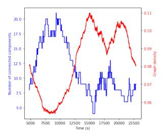
Fig. 4: Cross-evolution of the number of connected components and the graph density over a complete revolution around the Moon.
