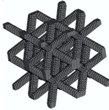
Fig. 10 Lattice structure voxelization, adapted from [74].
