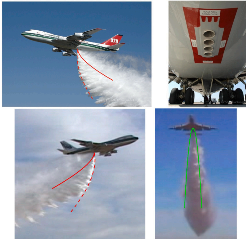
Fig. 17. Boeing 747 transformed into an airtanker dropping water. The exit is made of four circular holes of 40 cm in line. The water exit velocity is around 14 m/s and the aircraft velocity relative to surrounding air is approx. 70 m/s. The red line is relation (10), red dashed line is relation (10) with the prefactor K_y = 2.8 instead of K_y = 1.15 . The green line is relation (11). Photos in the first line: Courtesy of Marsaly (2016). Photos in the second line: Courtesy of Dan Reese President Global Supertanker Services from 2018 to 2021. . (For interpretation of the references to color in this figure legend, the reader is referred to the web version of this article.)
