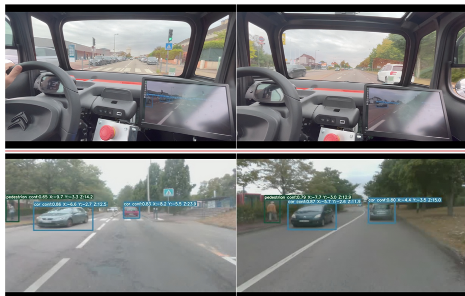
Figure 7. The algorithm tested in real-time conditions on an embedded Jetson.
