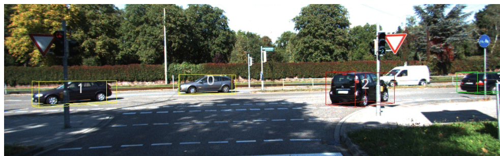
Figure 1. Object tracking with 3D bounding boxes and tracking numbers.
