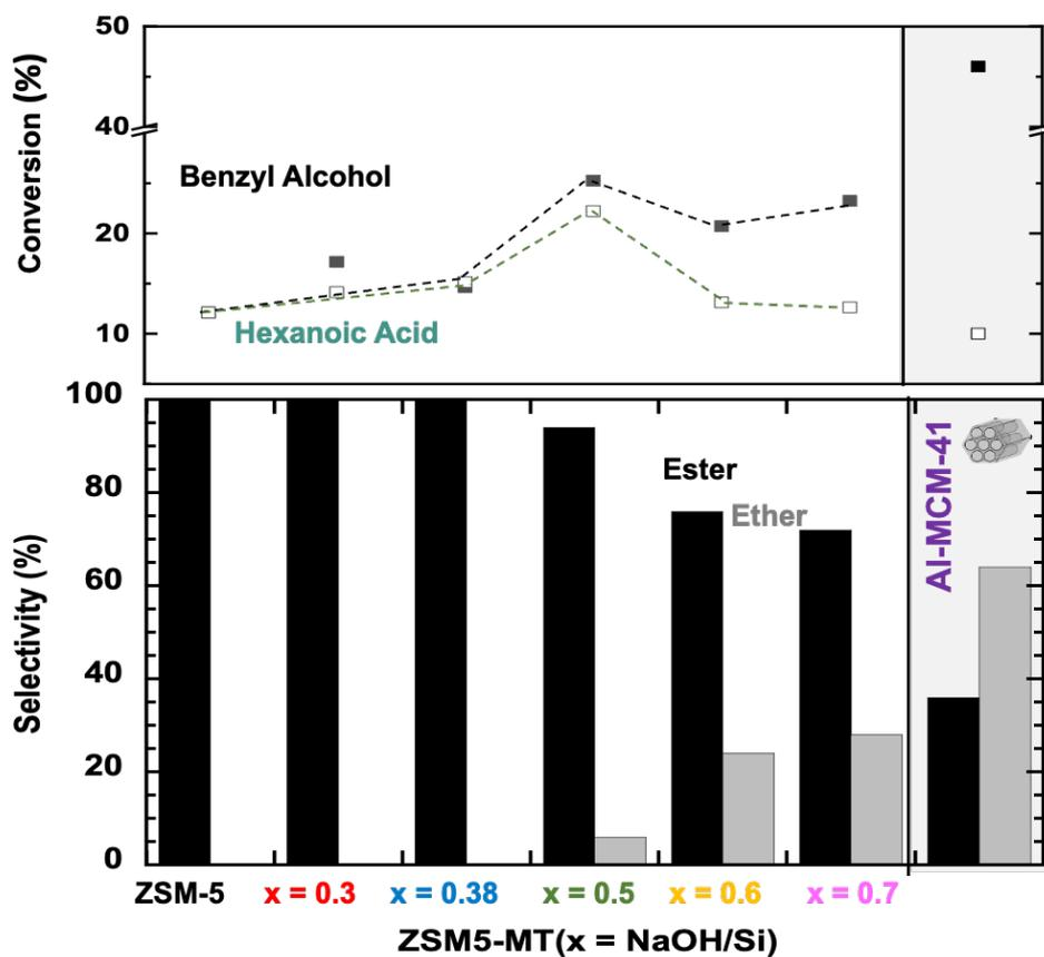
**Figure 7.** Esterification of benzyl alcohol by hexanoic acid with parent ZSM-5, ZSM5-MT(x) and Al-MCM-41 catalysts. (up) conversion of benzyl alcohol and hexanoic acid, (down) selectivity (black) in benzyl hexanoate and (grey) in benzyl ether.
