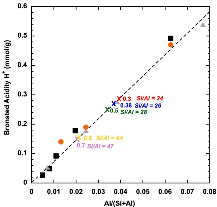
**Figure 5.** Relationship between the number of Brønsted acid sites in ZSM-5 catalysts of different Si/Al ratio as a function of their number of Al in the structure. The dashed line represents the fit of the data (Eq. 1). From the fit corresponding Si/Al ratio of ZSM5-MT(x) catalysts for  $x = 0.3, 0.38, 0.5, 0.6, 0.7$  have been calculated. Data from (orange circles) this work, (black square) from ref. 25, (grey triangle) from ref. 26.
