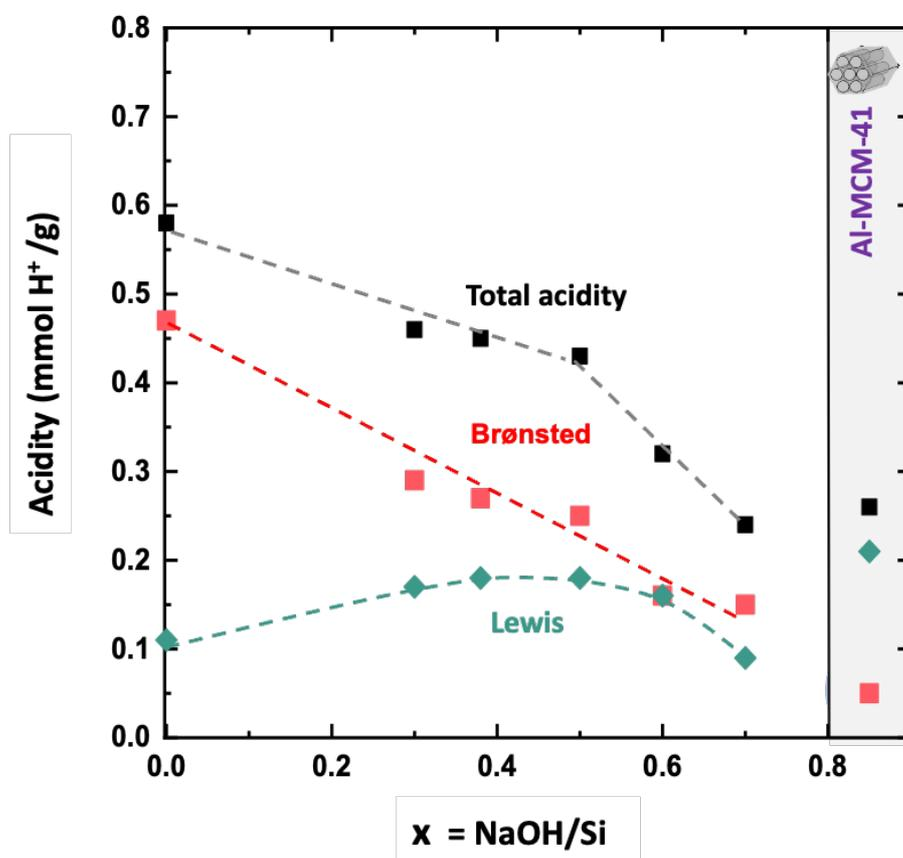
**Figure 3.** Evolution of the number of acid sites (Brønsted, Lewis, Total) determined by FTIR/pyridine (after outgassing at 423 K) as a function of x for ZSM5-MT(x). As comparison results for parent ZSM-5 (at x = 0) and Al-MCM-41 are given.
