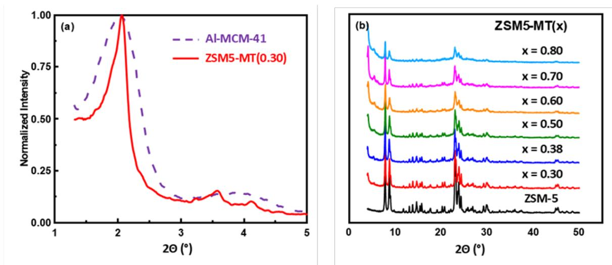
**Figure 1.** XRD pattern of ZSM5-MT(x) at (a) low and (b) large angles. As comparison XRD pattern of Al-MCM-41 and parent ZSM-5 are given. For sake of clarity, only low angle XRD pattern of ZSM5-MT(0.3) is given, the other ZSM5-MT(x) are shown in Figure S1.
