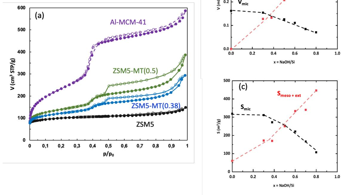
**Figure 2.** (a) Nitrogen sorption isotherms at 77 K of pristine ZSM-5, ZSM5-MT(x) and Al-MCM-41 (plain symbols for the adsorption and empty symbols for the desorption). (b) Micropore and mesopore volume and (c) micropore surface area and mesopore plus external surface area of ZSM-5-MT(x) determined by the corrected  $t$ -plot method. For sake of clarity, only isotherms of ZSM5-MT(x) with  $x = 0.38$  and  $0.5$  are given, the other isotherms of ZSM5-MT(x) are shown in Figure S1.
