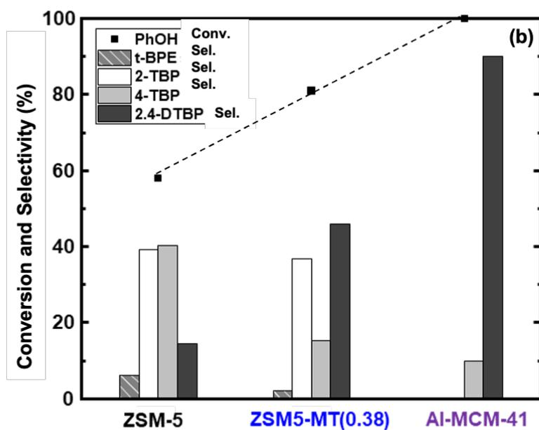
**Figure 6.** Results of the alkylation of phenol by *t*-BuOH over parent ZSM-5, ZSM5-MT(x) and Al-MCM-41 catalysts at 393 K. Phenol conversion for *t*-BuOH/phenol molar ratio of (blue square and dashed line) 3:1 and (red square and dashed line) 1:1. Selectivity of 2,4-DTBP for *t*-BuOH/phenol molar ratio of (blue bar) 3:1 and (red bar) 1:1.
