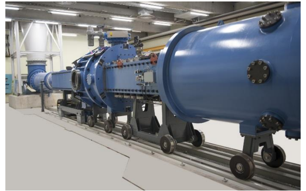
Figure 14. ISL's trisonic wind tunnel
