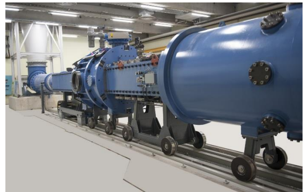
Figure 14. ISL's trisonic wind tunnel
