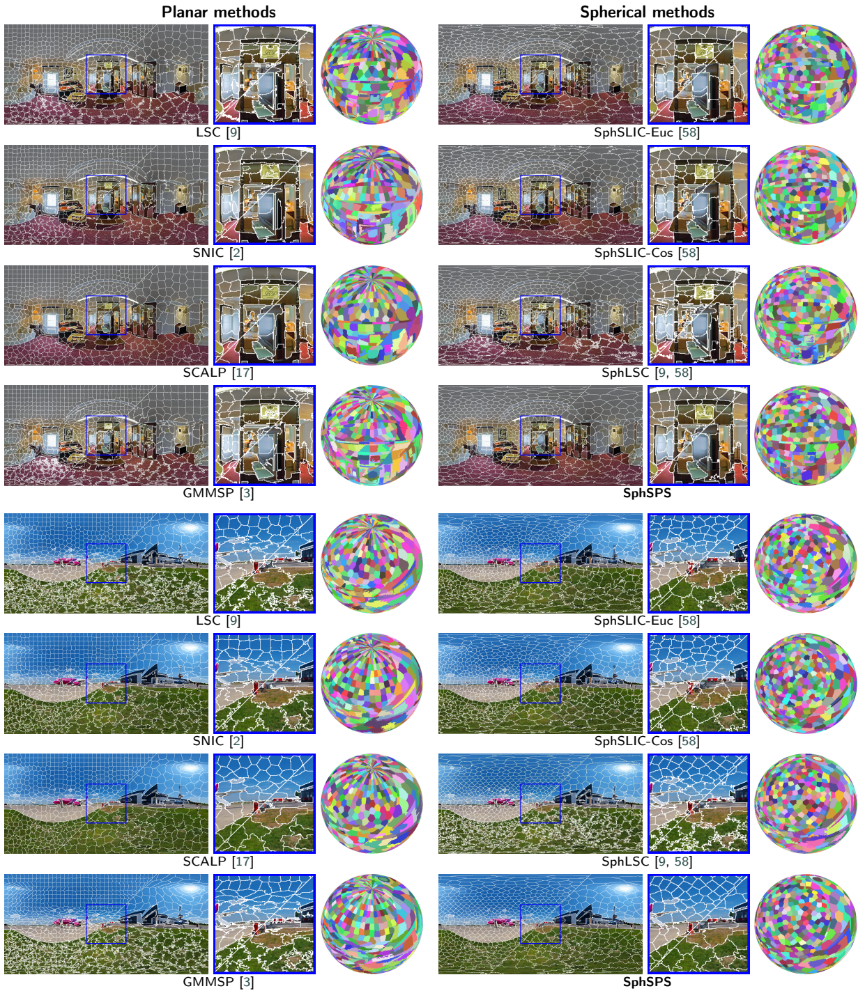
Figure 18: Visual comparison between SphSPS and the best planar and spherical (underlined) state-of-the-art methods on PSD images, for two superpixel numbers K = 1200 (top-left) and K = 400 (bottom right). SphSPS produces regular spherical superpixels with smooth boundaries that adhere well to the image contours
