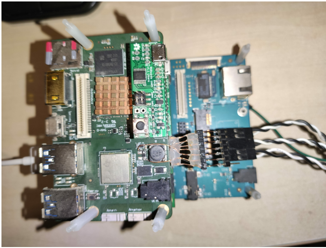
Fig. 9. Hikey960 board with power probe.
