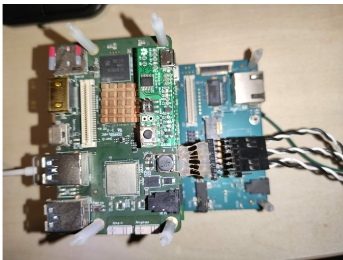
Fig. 9. Hikey960 board with power probe.
