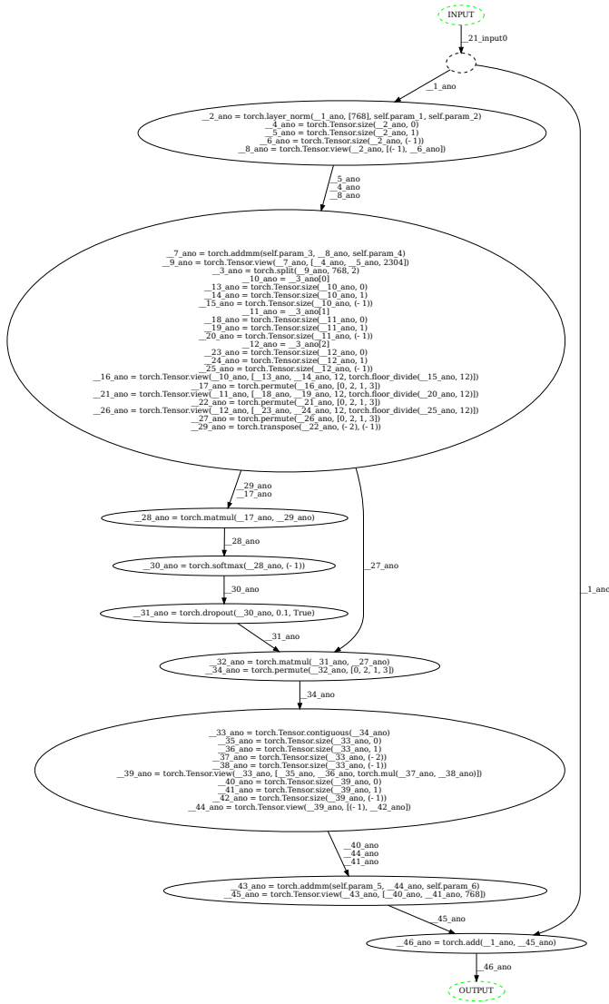
Figure 13. An anonymized version of an attention block from GPT2
