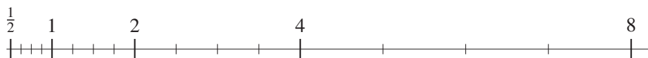
Figure 2.1. The FP numbers between 1/2 and 8 in the toy system \beta = 2 , p = 3 and infinite e_{\min} and e_{\max} .
