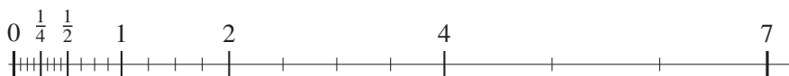
Figure 2.2. The positive FP numbers in the toy system \beta = 2, p = 3, e_{\min} = -2, e_{\max} = 2 .
